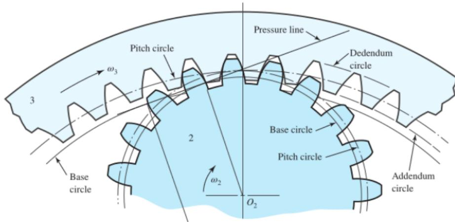
Note the location of the base circle of the internal gear.
