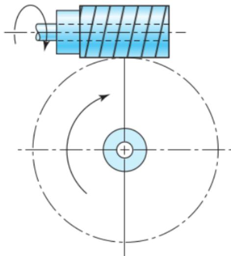
Worm gearsets are used to transmit rotary motion between nonparallel and nonintersecting shafts.
