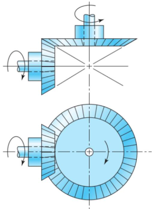
Bevel gears are used to transmit rotary motion between intersecting shafts.
