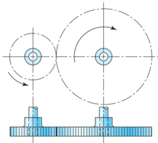
Spur gears are used to transmit rotary motion between parallel shafts.
