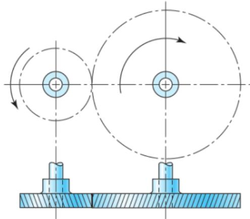
Helical gears are used to transmit motion between parallel or nonparallel shafts.
