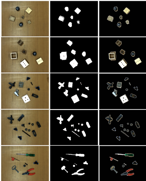
Fig. 3. (a) Original Image (b) Detected Salient Regions (c) Objects Present in Detected Salient Regions
