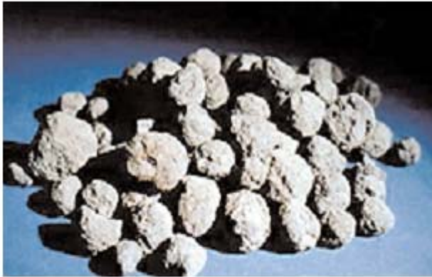
Fig. 2-9. Portland cement clinker is formed by burning calcium and siliceous raw materials in a kiln. This particular clinker is about 20 mm (¾ in.) in diameter. (60504)
