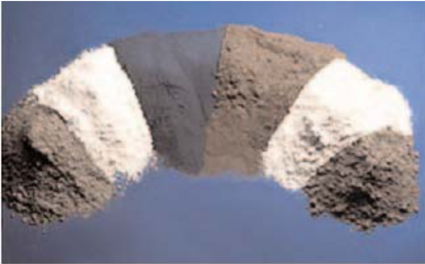
Fig. 3-1. Supplementary cementitious materials. From left to right, fly ash (Class C), metakaolin (calcined clay), silica fume, fly ash (Class F), slag, and calcined shale. (69794)
