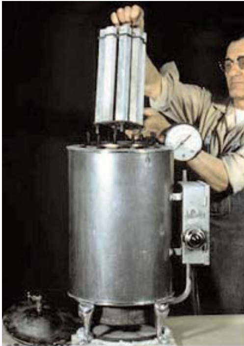
Fig. 2-35. In the soundness test, 25-mm square bars are exposed to high temperature and pressure in the autoclave to determine the volume stability of the cement paste. (23894)
