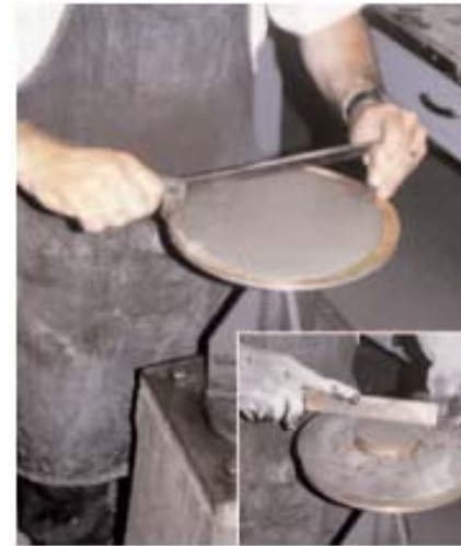
Fig. 2-37. Consistency test for mortar using the flow table. The mortar is placed in a small brass mold centered on the table (inset). For skin safety the technician wears protective gloves while handling the mortar. After the mold is removed and the table undergoes a succession of drops, the diameter of the pat is measured to determine consistency. (68821, 68822)
