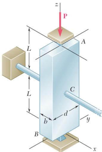
6. The steel bar AB has a square cross section. If it is pin connected at its ends, determine the maximum allowable load  $P$  than can be applied to the frame. Use a factor of safety with respect to buckling of 2. [13.51 kN]
