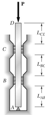
5. Column AB has a uniform cross section with  $b = 12$  mm and  $d = 22$  mm. The column is braced in the  $xz$  plane at its midpoint C and carries a centric load  $P$  of magnitude 3.8 kN. Knowing that a factor of safety of 3.2 is required, determine the largest allowable length  $L$ . Use  $E = 200$  GPa.
