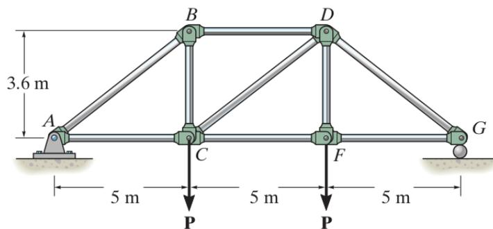
8. The truss is made from steel ( $E = 200 \text{ GPa}$ ) bars, each of which has a circular cross section with a diameter of 40 mm. Determine the maximum force  $P$  that can be applied without causing any of the members to buckle. The members are pin connected at their ends. [25 kN]
