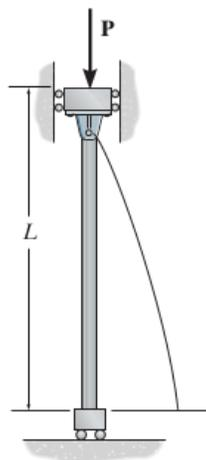
10. For a column with clamped-clamped conditions, the critical load may be determined by solving the fourth-order equation:
