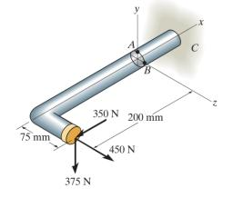
17. The thin-walled pipe has an inner diameter of 12 mm and a thickness of 0.6 mm. If it is subjected to an internal pressure of 3.5 MPa and the axial tension and torsional loadings shown, determine the principal stress at a point on the surface of the pipe.
