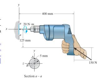
16. The 25 mm diameter rod is subjected to the loads shown. Determine the state of stress at points A and B.
