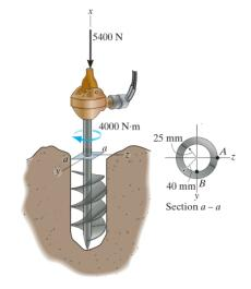
15. The drill is jammed in the wall and is subjected to the torque and force shown. Determine the state of stress at points A and B on the cross section of drill bit at section a-a.
