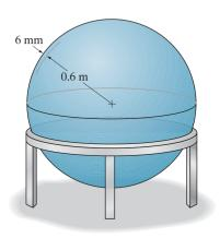
4. A thin walled spherical pressure having an inner radius r and thickness t is subjected to an internal pressure p. Show that the increase in the volume within the vessel is  $\Delta V = \frac{2p\pi r^4}{Et}(1-\nu)$ . Use a small-strain analysis.
