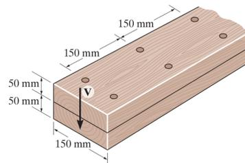
6. The boards are glued together to form the built-up beam. If the wood has an allowable shear stress of  $\tau_{\text{allow}} = 3$  MPa, and the glue seams at B and D can each withstand a maximum shear stress of 1.5 MPa, determine the maximum allowable internal shear force  $V$  that can be developed in the beam. [16.7 kN]
