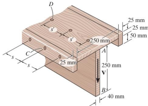
8. The beam is subjected to a shear of  $V = 2$  kN. Determine the average shear stress developed in each nail if the nails are spaced 75 mm apart on each side of the beam. Each nail has a diameter of 4 mm. [35.2 MPa]
