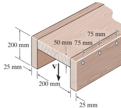
9. The beam is subjected to a shear of  $V = 800$  N. Determine the average shear stress developed in the nails along the sides A and B if the nails are spaced  $s = 100$  mm apart. Each nail has a diameter of 2 mm. [97.2 MPa]
