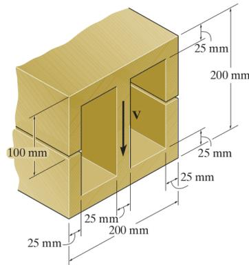
5. The beam is constructed from two boards fastened together at the top and bottom with two rows of nails spaced every 150 mm. If each nail can support a 2.5 kN shear force, determine the maximum shear force  $V$  that can be applied to the beam. [2.222 kN]
