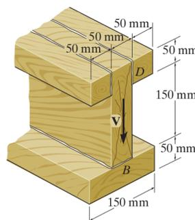
7. The beam is made from four boards nailed together as shown. If the nails can each support a shear force of 500 N, determine their required spacing  $s$  and  $s'$  if the beam is subjected to a shear force of  $V = 3.5$  kN. [ $s = 216.6$  mm,  $s' = 30.7$  mm]
