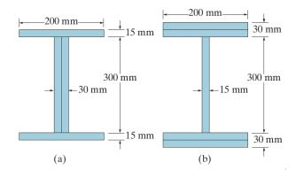
4. If the beam is subjected to an internal moment of M=3 kN·m, determine the maximum tensile and compressive stress in the beam. Also, sketch the bending stress distribution on the cross section.  $[\sigma_{\text{max,c}} = 14.94 \text{ MPa}, \sigma_{\text{max,t}} = 10.98 \text{ MPa}]$
