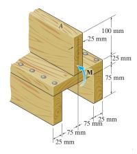
5. If the beam is subjected to an internal moment of M=100 kN·m, determine the bending stress developed at points A, B, and C.  $[\sigma_A=122 \text{ MPa (C)}, \sigma_B=51.1 \text{ MPa (T)}, \sigma_C=35.4 \text{ MPa (T)}]$
