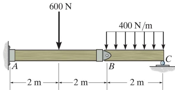
9. The compound beam is fixed at A, pin connected at B, and supported by a roller at C. Draw the shear and moment diagrams for the beam.
