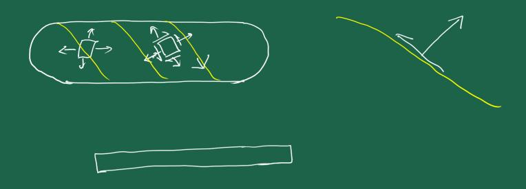
1. The thin-walled cylinder can be supported in one of two ways shown. If the piston causes the internal pressure to be 0.6 MPa, determine the state of stress in the wall of the cylinder for both cases. The inner diameter of the cylinder is 250 mm and the wall has a thickness of 6 mm. [(a) 12.5 MPa, 0 MPa (b) 12.5 MPa, 6.25 MPa]
