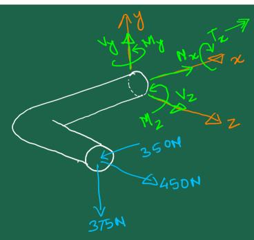
$$\sum_{z=0}^{z} f_{z} = 0 \Rightarrow V_{z} + 450N = 0 \Rightarrow V_{z} = -450N$$
