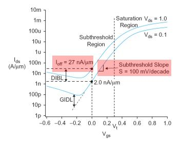
$$I_{ds} = I_{\text{off}} 10^{\frac{V_{gs} + \eta \left(V_{ds} - V_{dd}\right) - k\gamma V_{sb}}{S}} \left(1 - e^{\frac{-V_{ds}}{v_t}}\right) \qquad S = \left\lceil \frac{d \left(\log_{10} I_{ds}\right)}{dV_{gs}}\right\rceil^{-1} = nv_T \ln 10$$
