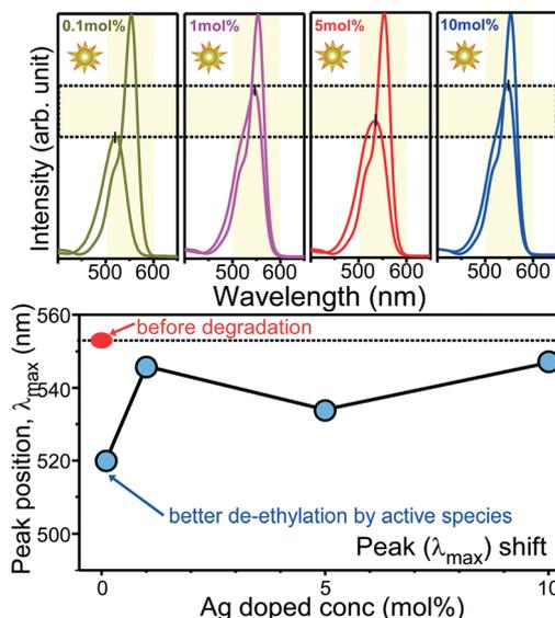
**Fig. 12** The photocatalytic degradation (and the change in peak position) of RhB over BiOI with Ag-loading under visible light irradiation for 6 hours. The UV-visible absorption peaks were normalized before photoirradiation.
