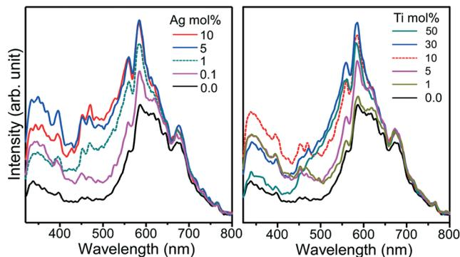
Fig. 8 The photoluminescence spectra of BiOI with increasing Ag (left) and Ti (right) loadings at an excitation wavelength of 280 nm.
