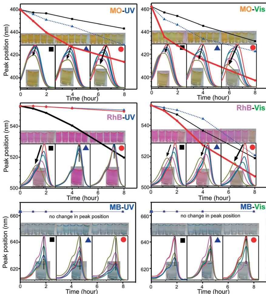
Fig. 10 Photodegradation (change in peak position and UV-visible absorption spectra) of the MO, RhB and MB solutions (10 mg L<sup>-1</sup>, 50 mL) by BiOI (■), 5 mol% Ag-loaded BiOI (▲) and 10 mol% Ti-loaded BiOI (●) under UV (left column) and visible (right column) light irradiation. The insets show the photos of the corresponding solutions with photodegradation time. The absorption wavelengths of the dyes (Fig. S6, ESI<sup>†</sup>) were omitted for clarity.
