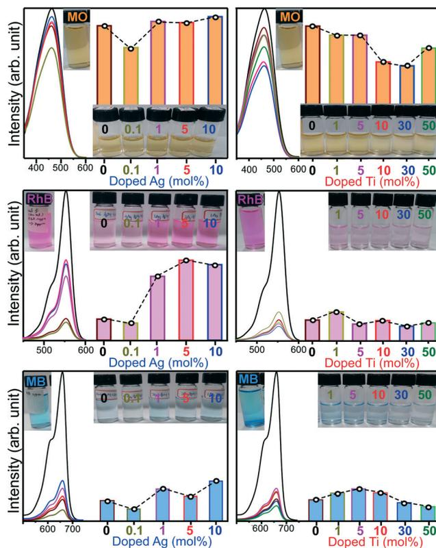
Fig. 9 The UV-visible absorption spectra and the corresponding peak intensities upon the adsorption of MO, RhB and MB ( $5\text{ mg L}^{-1}$ ,  $50\text{ mL}$ ) by 10 mg BiOI, Ag-doped BiOI and Ti-doped BiOI. The insets show the photo images of the corresponding dye solutions after adsorption. All the absorption peaks were normalized before adsorption.
