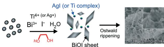
Fig. 3 A plausible growth mechanism of the echinoid-like Ag and Ti-loaded BiOI nanostructures.
