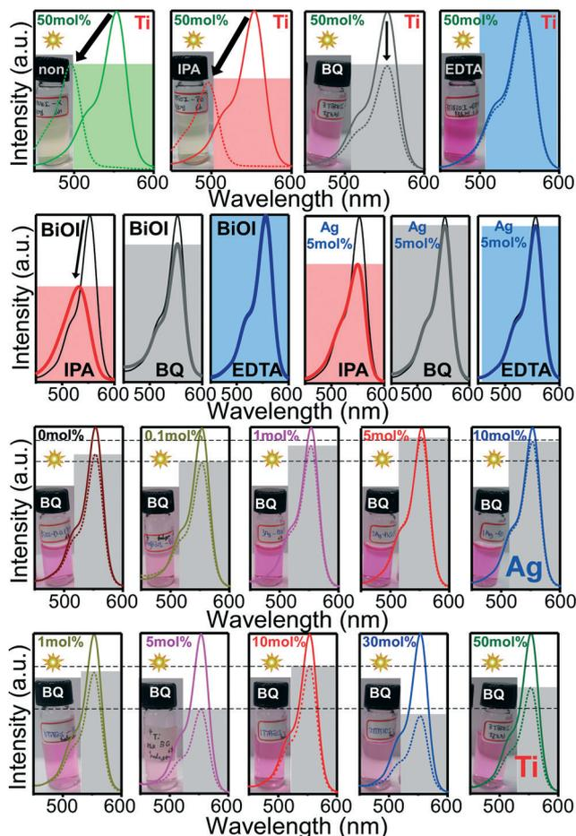
**Fig. 11** The photocatalytic degradation (top two lines) of RhB with BiOI, Ag(5 mol%)-BiOI and Ti(50 mol%)-BiOI in the absence and presence of scavengers (IPA, BQ and EDTA) under visible light irradiation for 6 hours. The photocatalytic degradation (bottom two lines) of RhB over Ag-BiOI and Ti-BiOI with different Ag and Ti-loaded BiOI in the presence of BQ under visible light irradiation for 6 hours.
