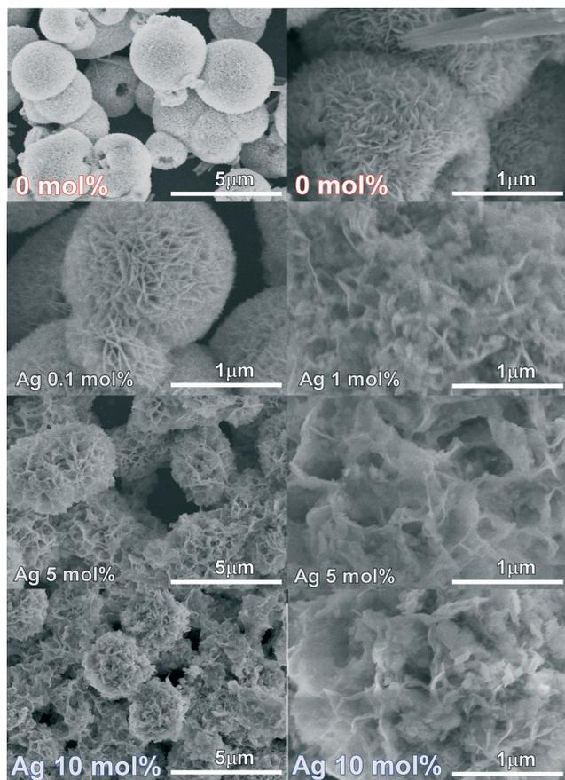
Fig. 1 SEM images of BiOI doped with different concentrations (0.1, 1, 5 and 10 mol%) of Ag.
